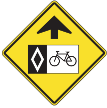
Reserved bicycle lane ahead
